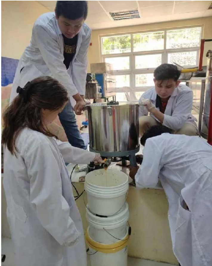
Students from the Don Mariano Marcos Memorial State University-Mid La Union Campus test the Beeswax Capping Spinner prototype that can improve the way honey is processed by beekeepers. CONTRIBUTED PHOTO
