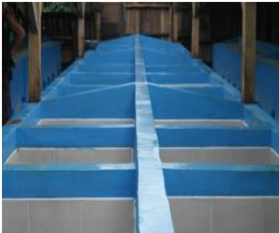
Coagulating and aging tank provided to Maasin Rubber and Coco Farmers Association by DTI-9 thru SSF Project
